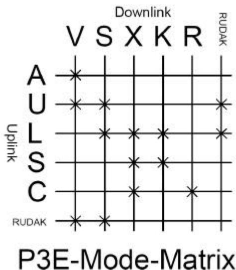
Figure 7: The Mode Combinations, as they are planned for P3E. At publication time the noted option for 29 MHz (A-band) and RUDAK was not included.
