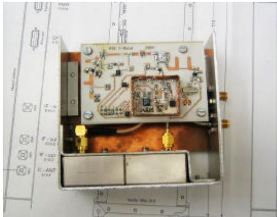
Figure 6: A first construction sample of the C-band receiver shows the compact construction (left under the filters).
