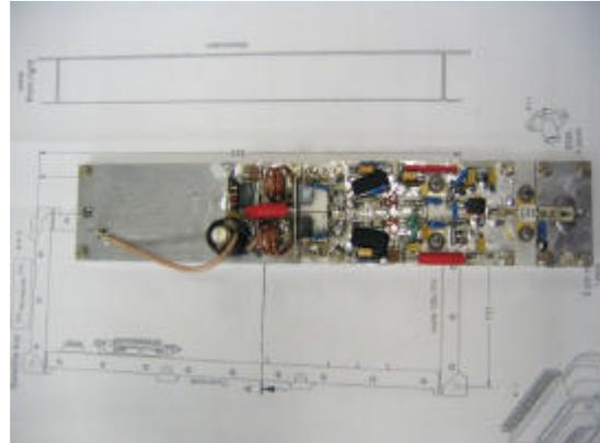
Figure 3: The operational sample construction of the 2-meter final stage power amplifier.
