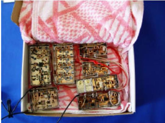
Figure 4: Transponder in a box – The individual modules (local oscillators, mixers, amplifier stages, and IF) of the U/V transponder.
