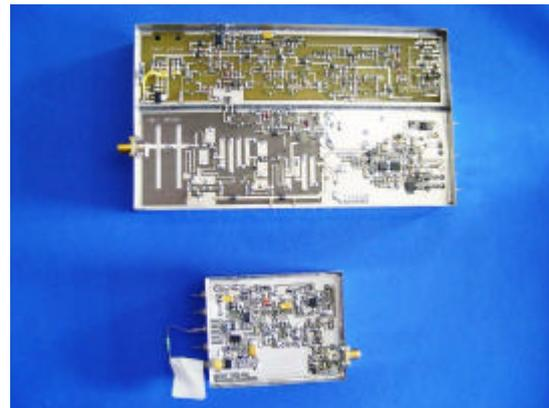
Figure 5: The L-band receiver (upper) and the command receiver (lower) for P3E.
