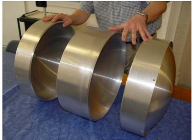
Fig. 2: Three pieces form two chambers of the tank.
