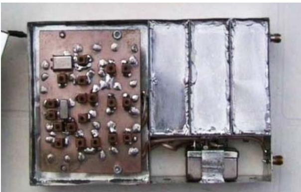
**Fig. 7:** The U/V transponder: at left the TX board, upper right 70 cm input filter, lower right the 100 kHz wide IF filter. Below the TX the RX board is located.
