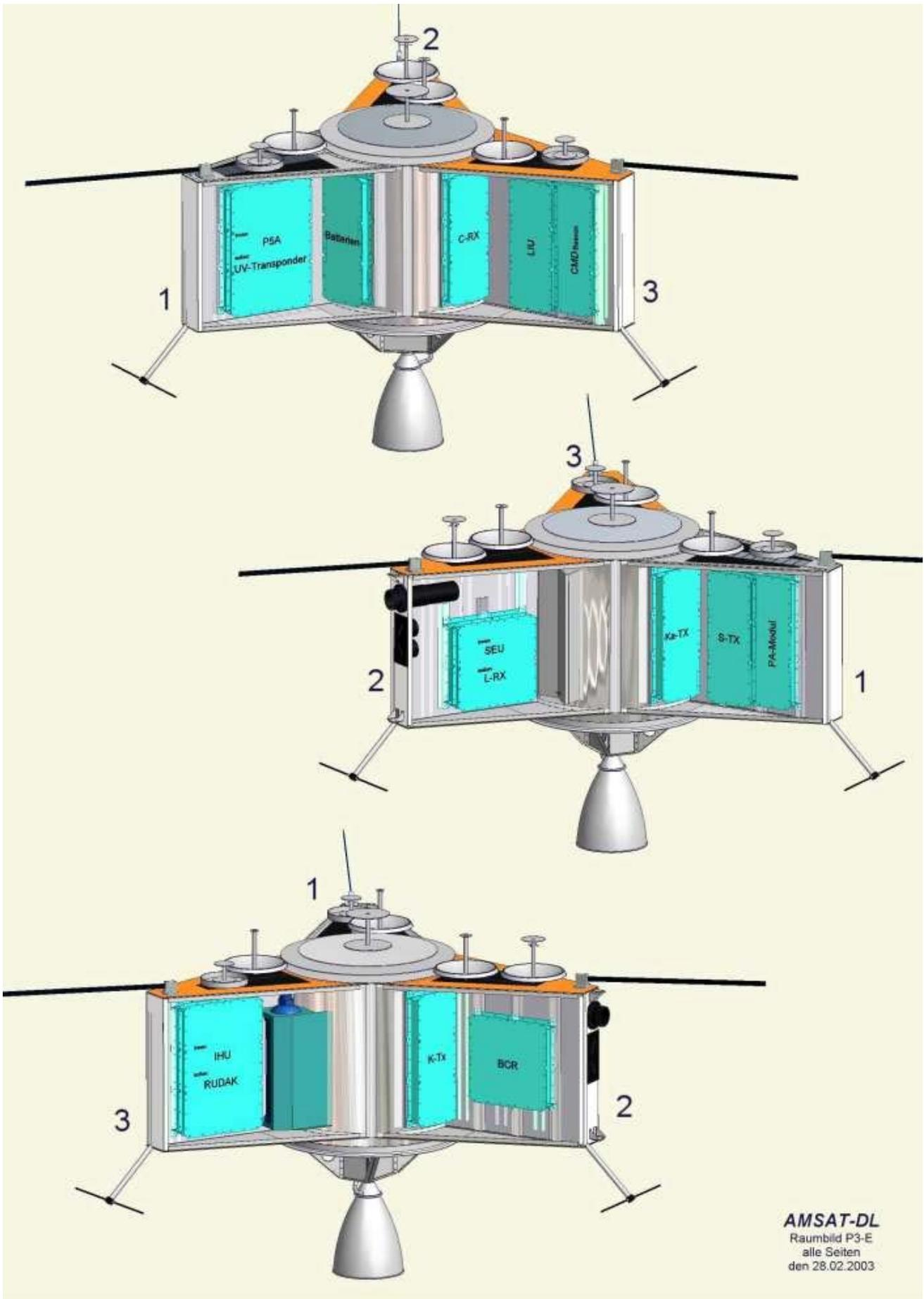
Fig 8: View into the different sections of P3E
