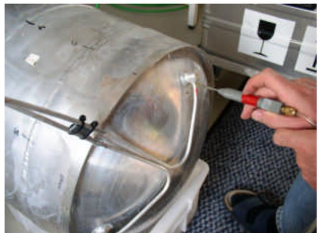
*Figure 7: The last integrity test of the tank's end.*
