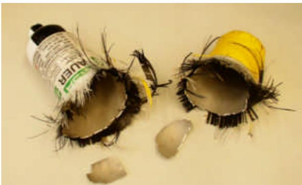
*Figure 4: The helium flask burst at 1600 bar, it has to withstand 400 bar on board P3E.*
